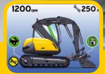
A new TFT colour screen makes the control panel very easy to use. Regardless of brightness, the operator can easily view all useful information: mode currently being used, speed, engine speed, number of hours, cylinder selected, safety features activated.
