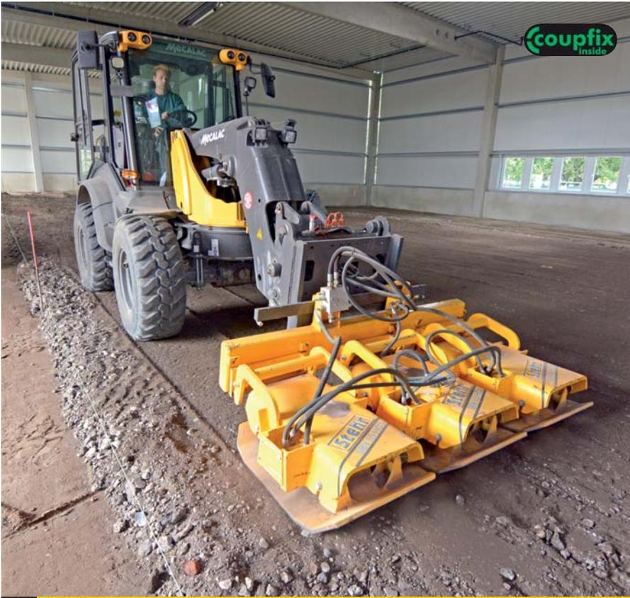
▲ The hydraulic system of the AS 900 comes optimally matched to our levellers ex factory.
