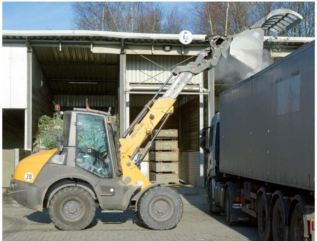
➔ With a load over height of 4.67 m, the AT 900 easily loads trucks with high sides
