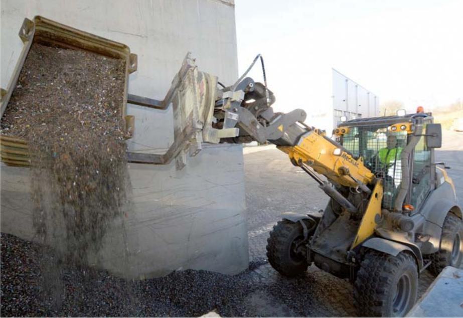
→ Equipped with a box rotator, the AT 900 handles heavy boxes filled with raw material
